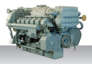
12-cylinder, 4-stroke, water-cooled diesel engine, with direct-injection, turbocharger, air-cooler, built-up heat exchanger and sea water pump.
