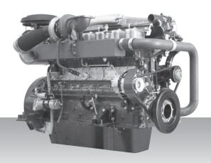
6-cylinder, 4-stroke, water-cooled diesel engine, with direct-injection, turbocharger and air-cooler.
