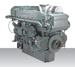
6-cylinder, 4-stroke, water-cooled diesel engine, with direct-injection, turbocharger, air-cooler, built-up heat exchanger and sea water pump.
