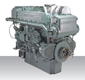
6-cylinder, 4-stroke, water-cooled diesel engine, with direct-injection, turbocharger, air-cooler, built-up heat exchanger and sea water pump.
