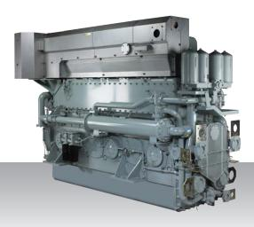
6-cylinder, 4-stroke, water-cooled diesel engine, with direct-injection, turbocharger and air-cooler.
