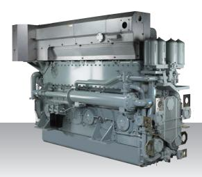
6-cylinder, 4-stroke, water-cooled diesel engine, with direct-injection, turbocharger and air-cooler.
