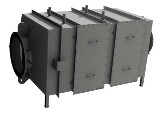
To comply with the IMO Tier III regulations, an average NOx reduction of 75% is needed compared to the IMO Tier II regulations. To meet this reduction, an after-treatment system is needed. Mitsubishi Marine Engines and Generator Sets can now be equipped with a Selective Catalyst Reduction (SCR) system. An SCR system is a system that reduces NOx emissions from the engine exhaust gases.
